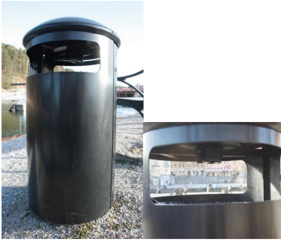
Figure 10 The sensors are installed inside at top of the litter bins.
